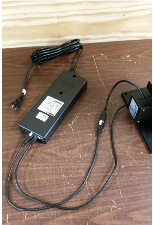
Connect lift motor cable to motor extension cable, then connect extension cable to port 1 on control box.
